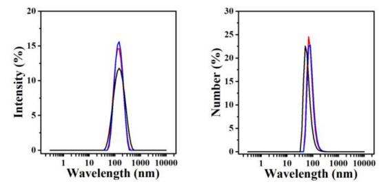
As shown in the figure, the hydrodynamic size of PVP modified ZnO<sub>2</sub> nanoparticles is larger than the TEM size.
