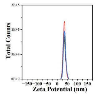
It can be seen from the figure that the Zeta potential of PVP modified ZnO<sub>2</sub> nanoparticles is 36.17 mV.
