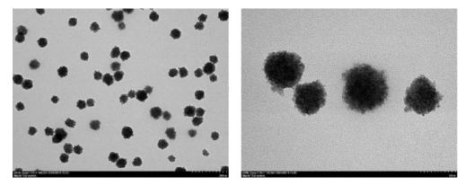
The above figure shows that zinc peroxide nanoparticles are uniformly dispersed with a size of approximately  $40 \sim 50$  nm.
